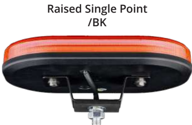
Raised single point fixing to increase height by 38mm.
